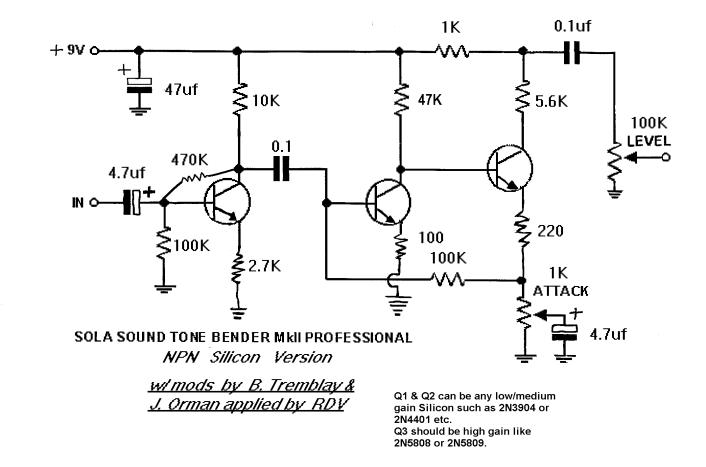
The Q3 5.6k collector resistor can be changed to a 10k trim-pot for Tweaking. Best results are at 4.5 to 5.5v measured at Q3's collector to Ground.
